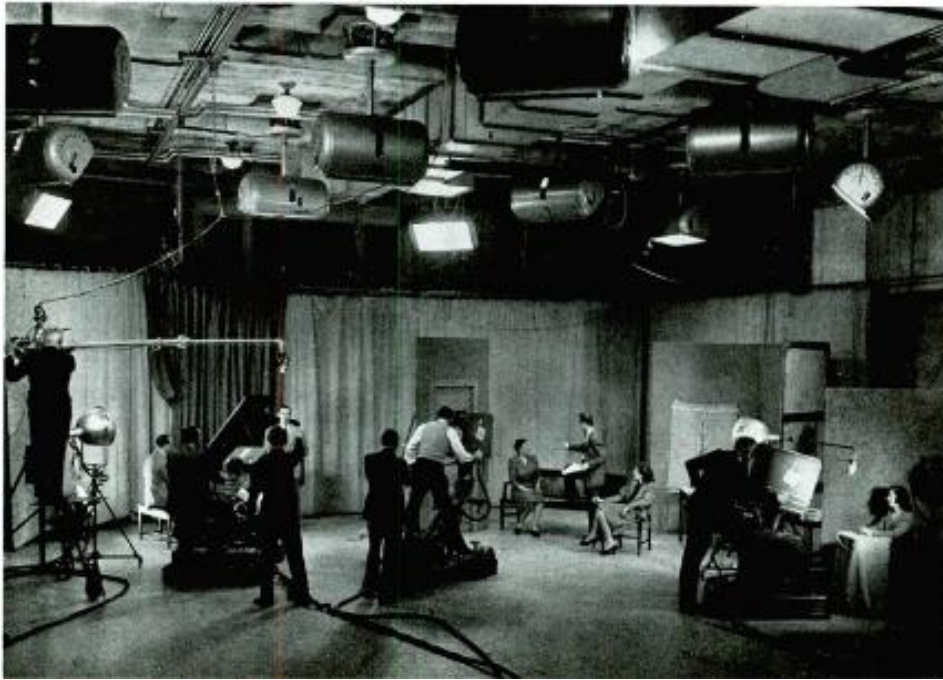
Station WRGB in action. Note the three cameras in use. Also note the overhead mercury vapor lights. (General Electric Photo.)
